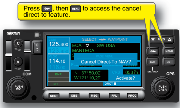
Figure 3-24. Canceling a direct-to operation.
